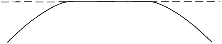
Fig. 10.6.5. A curved crystal merging with a flat crystal facet below its roughening transition. The curved surface has a power-law singularity of the form \tilde{h}(\tilde{x}) = \tilde{h}_0 - A(|\tilde{x}| - \tilde{x}_0)^{3/2} .
